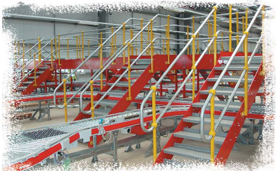
Conveyor bridges and walkways
